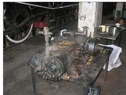
S09 - Stoker motor on the bench. It looked OK on the outside but ran quite poorly.
