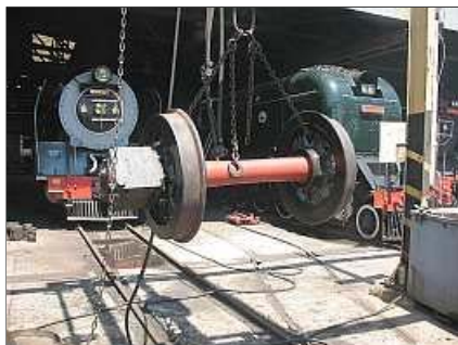
S07 - The overhauled donor Bissel axle with a full set of new bearings is being hoisted to the work area with Lyndie Lou's coal bunker poking out into the sun at the rear right.
