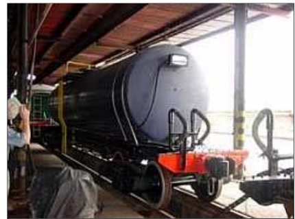
R03 - Lyndie Lou's water canteen has just been cleaned and all auxiliaries and fittings repainted. Note the fitted double-beam headlamp for operation in reverse.
