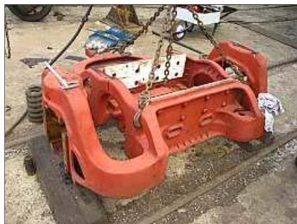
S08 - The stripped, cleaned and primed Bissel truck frame clearly shows the use of maintenance-free Vesconite as a modern bearing material for the bolster plate slides.
