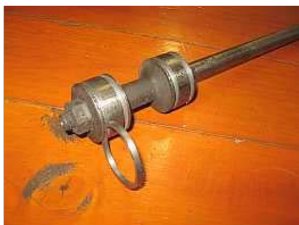
S10 - A test fit of a newly fabricated valve ring, still warm from the lathe, into the grooves of a cleaned valve spool.
