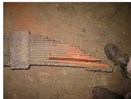
S15 - One axle spring with a broken leaf that fell completely out upon removal. And even in the small photograph, you can clearly see a second broken leaf two leaves up from the gap.
