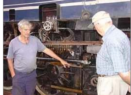
R06 - Team leader of Lyndie Lou's second refurbishment work, John Dadford (Left), talks to Wolf Mensing of Rovos Rail, as they examine the nearly completed GMAM locomotive. (Visible to the right of John's head is the manual priming wheel for the newly serviced mechanical lubricator.)
