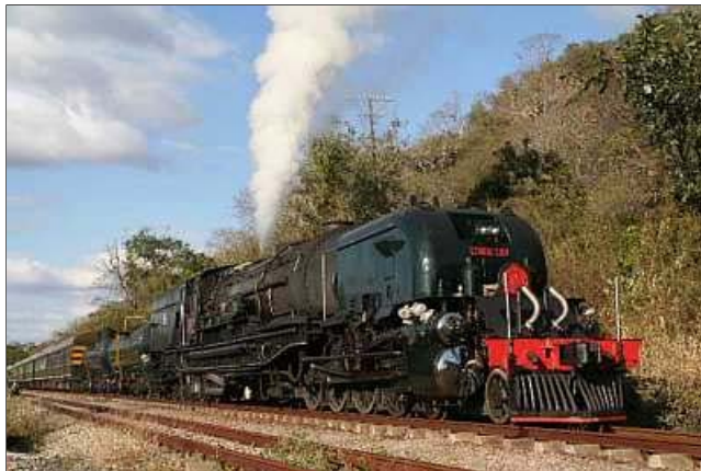
R07 - A newly repainted Lyndie Lou during a strenuous debut run in the eastern Transvaal. Note the CLEAN stack and the blowing safety valves. Photo by Chris A. Janisch (Friends of the Rail)
