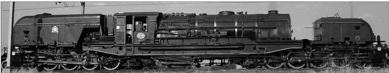
S02 - The side view of the real thing. This is a desaturated Rovos-era colour photo to better match Sue Lawrence's drawing above. This is the RHS of the locomotive and differing details include the Reverser, Brake Discharge line, Drifter Valve, Mechanical Lubricator on the front unit and the Mechanical Stoker visible inset into the coal bunker. (Pic by Colonel Andre Kritzing)
