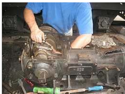
S11 - An experienced ex-Millsite Railways fitter is up to the elbows in a full rebuild of Lyndie Lou's stoker engine.
