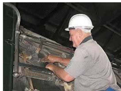
S12 - An old railway man faces the tedious task of removing the paint from the brass and copper work.
