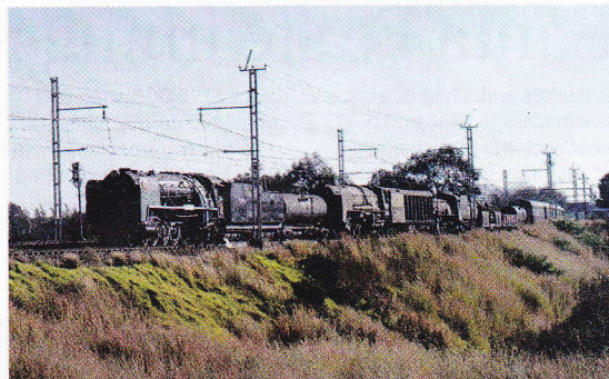
↑ David Shepherd's '15F' 4-8-2 No. 3052 leads condensing Class 25 4-8-4 No. 3451 and '19D' 4-8-2 No. 2540 out of Millsite on June 19. AIDAN McCARTHY
