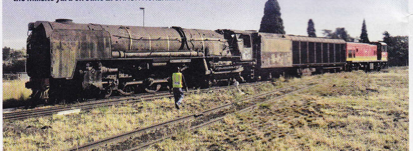
South African Class 25 condensing 4-8-4 No. 3451 is dragged out of the Millsite yard on June 2. SHAUN ACKERMAN
