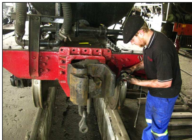
P06 - Bossy the Tanker got a new coupler cut cable fitted. The clevis bolt had seized, so after some fruitless battles with spanners, they 'cooked' the bolt off with alternate torching and then quick-quenching with cold water.
