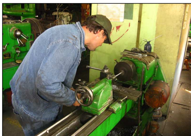
P08 - Meanwhile, Dawie is seen machining a new Die Block Locking Pin from rod stock that was slightly oversized. For some reason, Midas Motor spares don't stock 15F parts. Very inconvenient...
