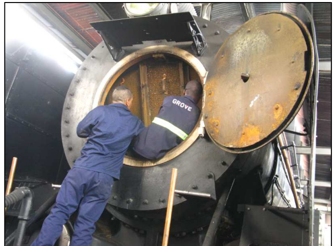
P02 - We have a new batch of Africa Academy Appies to torture ... I mean ... train up. This likely bunch were tasked to put 15F 3046's smokebox and arrestors back together again. It was dismantled and left partially open through the quiet months of December to dry out after cleaning.
