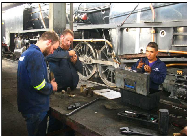
P05 - A little later and the Appies are seen busy cleaning and copper-greasing the conical threaded washout plugs to be put back in. They might be doing coach lifting next week!
