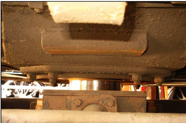
P02 - The main point of coach LIFTING is to disconnect the bogies, and to jack the coach up over the bogies for inspection of the pivot and its bearings. With the 40-ton coach being jacked up on both sides, you can see the shiny bolster pivot lifting away from the bearing boss right in the center of the picture. All the other jobs can usually be done with the coach resting on its wheels as normal.
