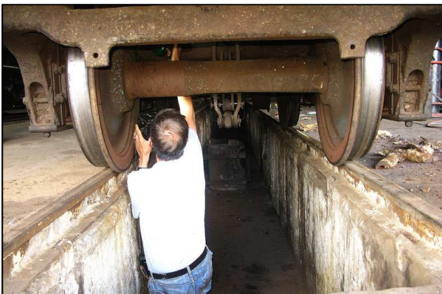
P04 - Coach lifting time is also used to give the brake linkages and suspension gear a good old-fashioned oil round. Here, Nicholas Goodale gets to work to lubricate the numerous pinned brake linkages and pivots.
